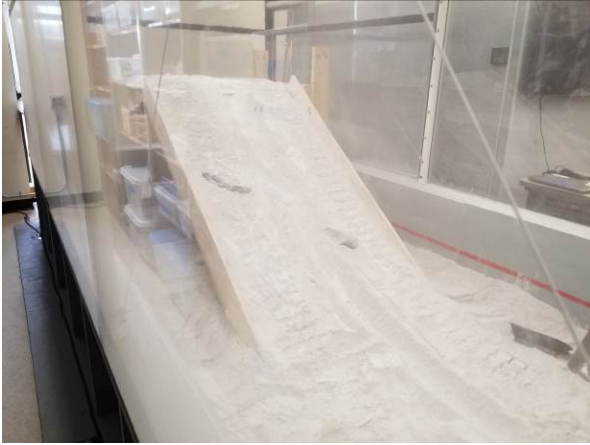
Figure 3: Simulant “sandbox” used for vehicle testing
